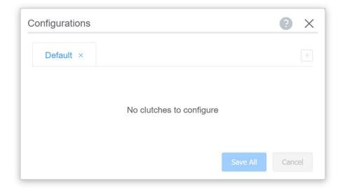
**HINT:** To define a load case, as shown later, a configuration must be defined even if no clutches exist.
