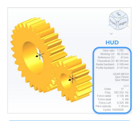
**HINT:** Gear or gear mesh *order*, as shown in HUD, is based on the reference part in Settings, from the Analysis ribbon.
