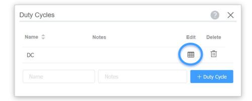
**HINT:** A *duty cycle* is a collection of *load cases*, i.e. discrete loads, preferably binned from real-world time series data.
