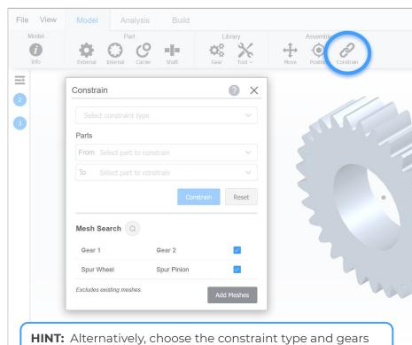
**HINT:** Alternatively, choose the constraint type and gears from the dropdown menus, then click **Constrain**.
