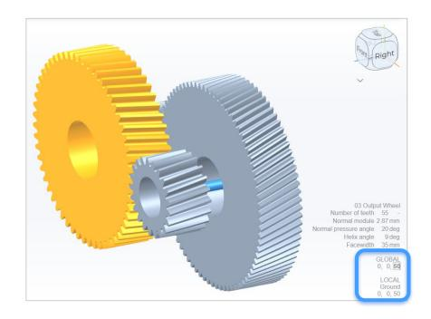
**TIP:** Ctrl + click two gears in 3D Viewer to see valuable information in the bottom right, including if the gears are "meshable" and the center distance for no backlash.
